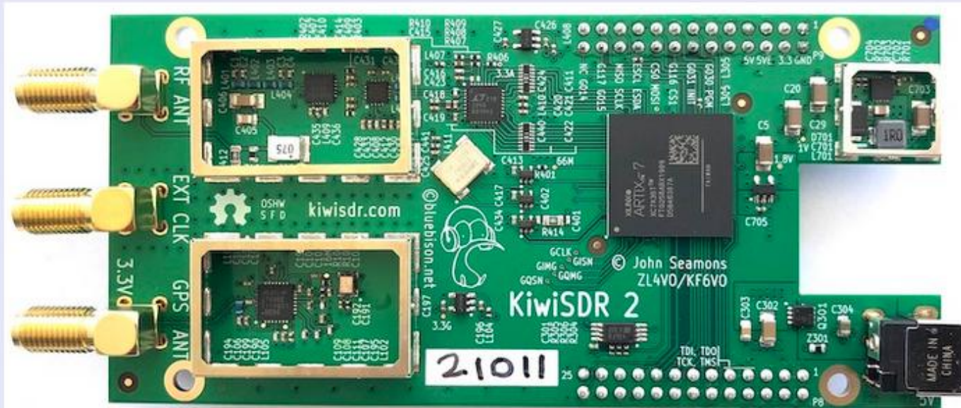
KiwiSDR: Wide-band SDR + GPS cape for the BeagleBone Black
